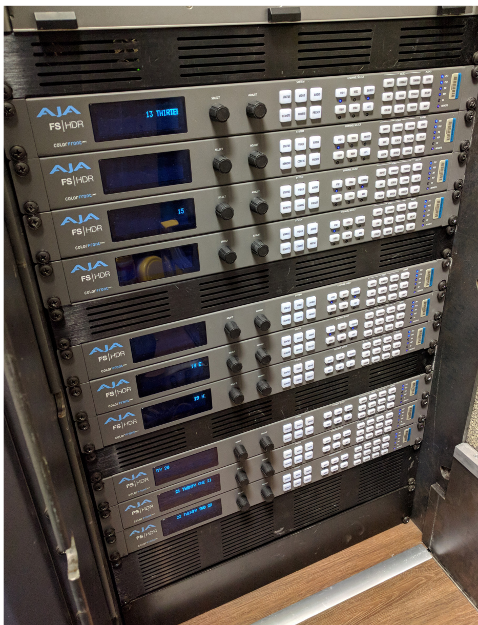
The new Mobile TV Group 4K HDR Double Expando is equipped with 14 AJA FS-HDR frame sync/HDR converters.
