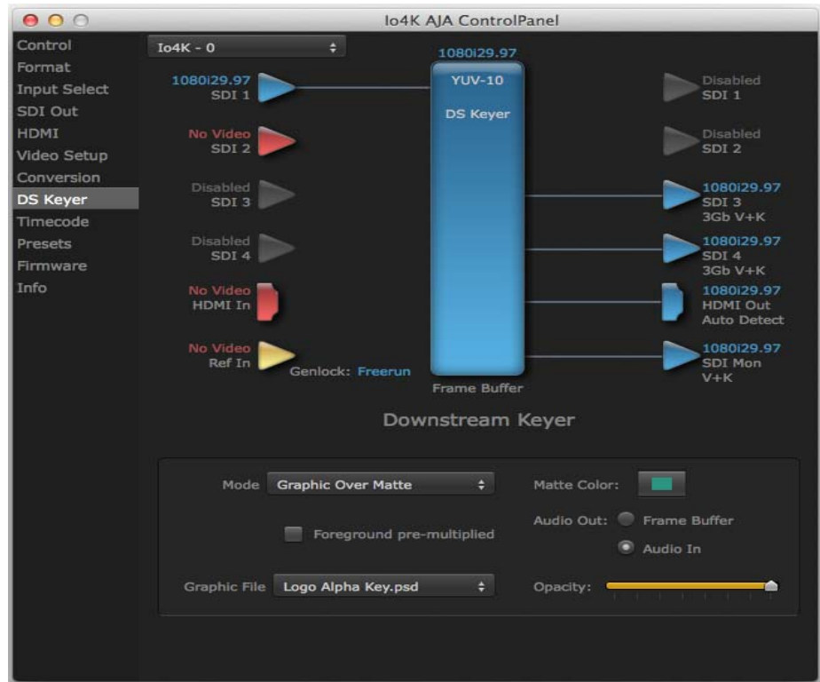
Figure 38. AJA Control Panel, Downstream Keyer Screen
